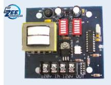
**78820** Replacement board for Kleen Flo®, Delaval® or Surge® air injectors
